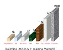
On the contrary to the materials such as concrete, gas concrete, etc. used in the walls of the structures, the polyurethane-filled sandwich panels meet the same thermal insulation and their thickness is smaller. Therefore, the area and volume within the building can be expanded in a measurable manner.
