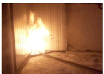
The contribution of the material in the expansion of the fire, even the resistance shown by the material against the fire which is also qualified as flammability capacity is called fire performance. A panel system formed of inflammable metal surface as well as polyurethane can be qualified as B,s2,d0 i.e. hard to burn according to EN 13501 norm, however evaluating the behavior of the fire to occur in the building over the fire performance of the wall coating material will be incomplete.
